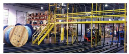
Service loops are completed at our 100,000 sq. ft. manufacturing facility in Houston, Texas. Cable bundles are inserted in a protective hose and fully potted.
